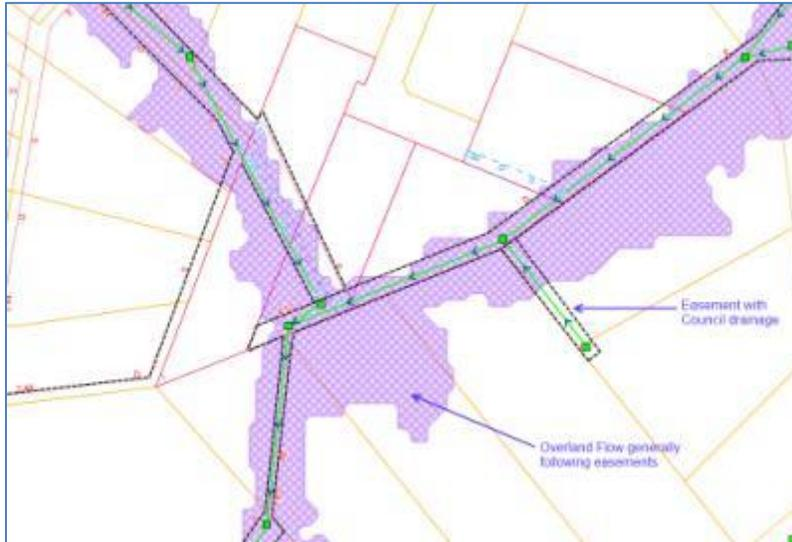
Figure 8 - Council's flood modelling outputs showing an overland flow path, generally following the alignment of easements
