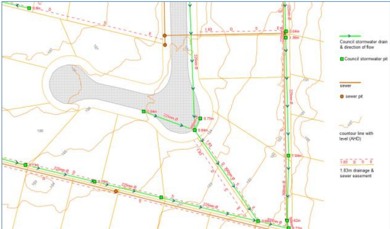
Figure 3 -- A typical snapshot from Council's GIS asset layer showing easements, Council drains and pits, contour information and sewer
