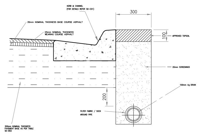
SUBSOIL Ag. DRAINAGE PIPE TRENCH DETAIL
