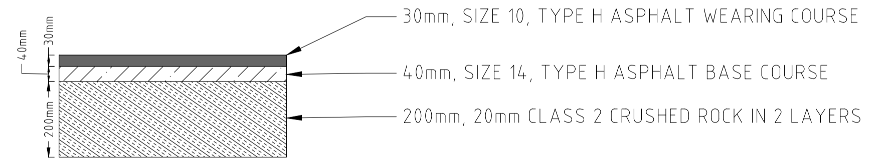
PAVEMENT DETAIL NTS
