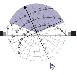
Eastern facades are exposed to solar heat gains just as much as western facades, only we perceive it as less as the ambient temperatures are cooler in the morning. All this is important to consider, particularly when designing sun shading for different facades.
